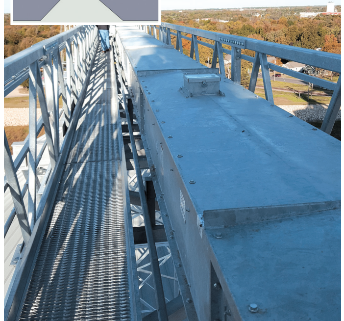
Hip Style Bolted Conveyor Covers Patent No. 8,047,358
